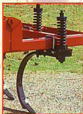
Dent standard Standard tines Standard Zinken
